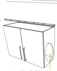
For safety reasons, it is critical that all wall cabinets are anchored with at least one screw (not provided) passing thru the lower inside back panel of the cabinet and onto the wall.
